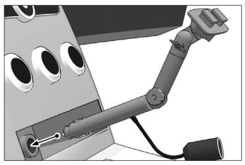
Insert device into holder by pushing down on the lower support legs; use power dongle with a separate 12V car charger (not included) to charge device. Adjust arm position as necessary.
