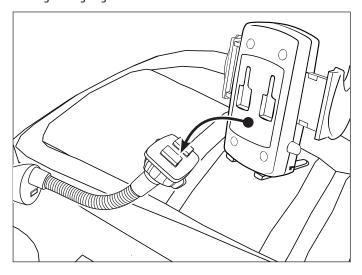
3 Insert device into Mega Grip holder and secure by squeezing the spring-loaded arms together. Release device by pressing release button.
