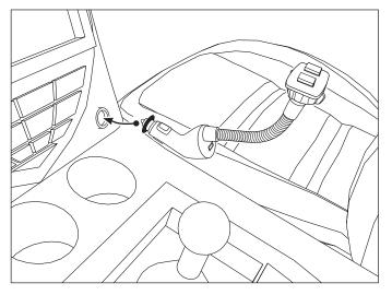
2 Attach Mega Grip holder onto the dual T-Tabs and secure with tightening ring.
