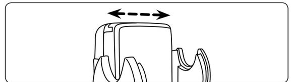
**!** Use caution when adjusting the swivel head. Use caution when inserting or removing the pedestal or the phone from the holder. Make sure that the teeth of the vent clips are open wide enough to not damage the vent fins / blades.
