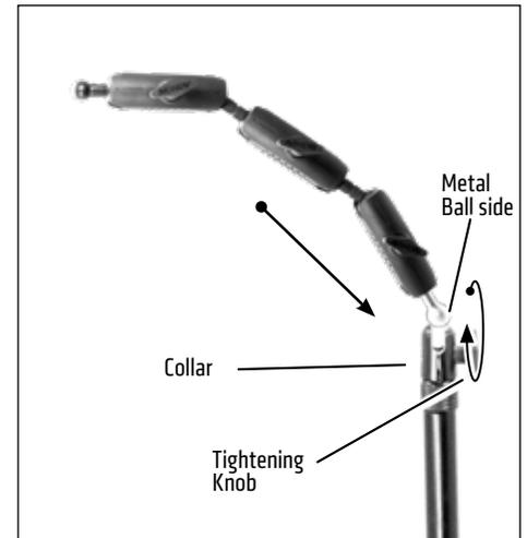
**3** Unscrew tightening ring from holder. Place ring over the 17mm end of mount then snap the holder onto the ball. Set to desired position, then tighten ring.
